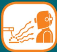
**PROTECT** your eyes and face with a properly-fitted welding helmet and with proper grade of filter plate (See ANSI Z49.1).
