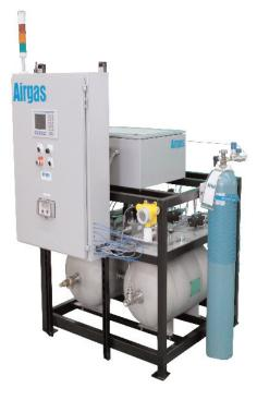
**Description:** The Airgas Tri-Mix Blender is designed for customers utilizing carbon monoxide mixtures for meat packaging operations. The mass flow controller based system is capable of producing a 4000 ppm carbon monoxide, 35% carbon dioxide balance nitrogen mixture that is evaluated by an integrated process analyzer.
