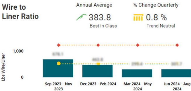
Figure 4: This customer has managed to improve their wire-to-liner ratio during the past 12 months by establishing a regular schedule that calls for changing out their liners more frequently.
